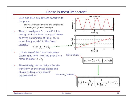
In principle DLLs and PLLs are sensitive to phase only. Some times, depending on the type of the phase detector, they are also sensitive to the signal amplitude. This is however an undesirable feature and, as a rule, should be minimized or, if possible, eliminated altogether.
